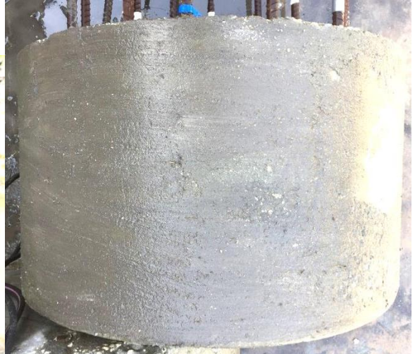
Figure 3.11 Shaft 11: f'_c 4530 psi; drilled shaft mix; 65 sec/qt polymer; smooth; no creases
