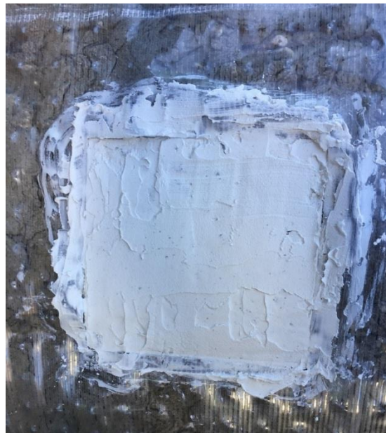
Figure 3.33 Testing template filled to approximate a void free surface
