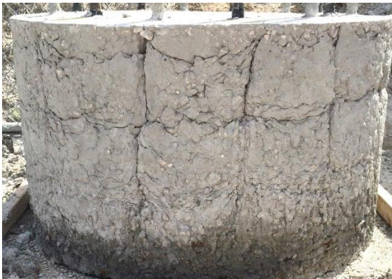
Figure 3.21 Shaft 21: f'_c 4100 psi; drilled shaft mix; 42 sec/qt bentonite; rough; well-defined creases
