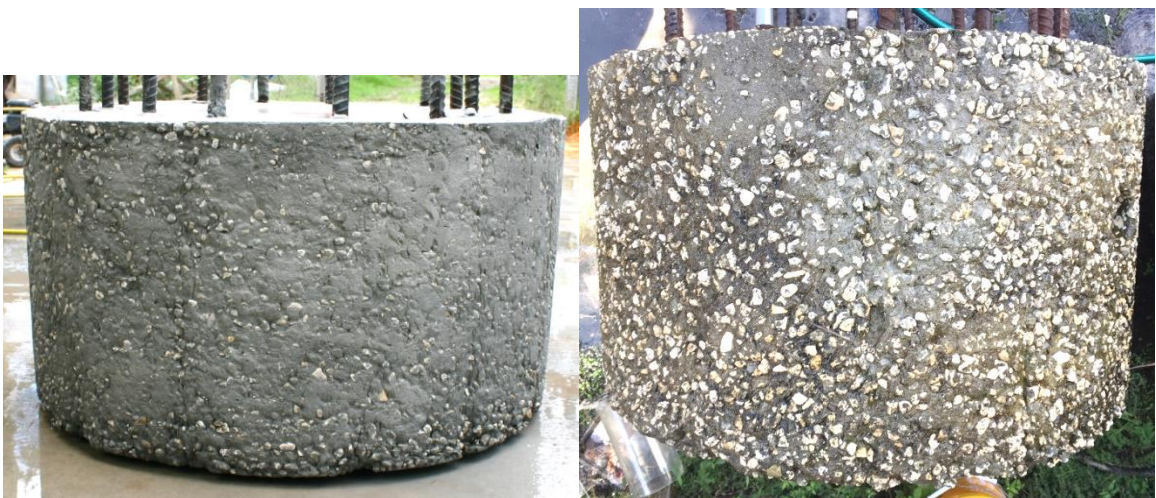
Figure 3.6 Shaft 6: f'_c 4358 psi; drilled shaft mix; water cast; smooth; faint channeling.
