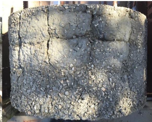
Figure 3.21 Shaft 21: f'_c 4100 psi; drilled shaft mix; 42 sec/qt bentonite; rough; well-defined creases
