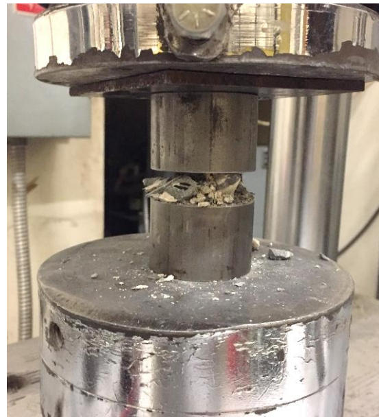
Figure 3.83 Core sample undergoing compressive strength testing
