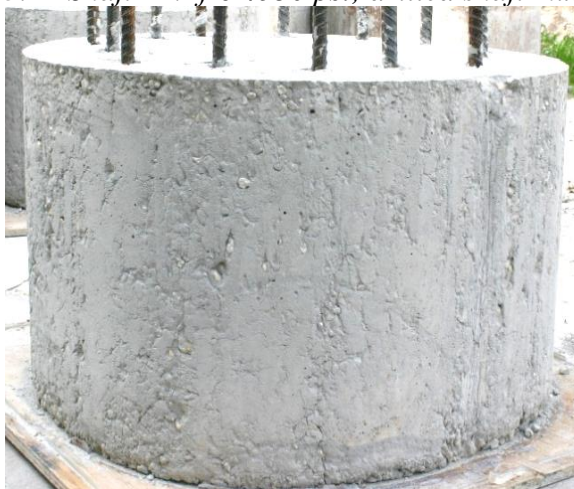
Figure 3.13 Shaft 13: f'_c 4753 psi; drilled shaft mix; 30 sec/qt bentonite; coarse; faint to no creases
