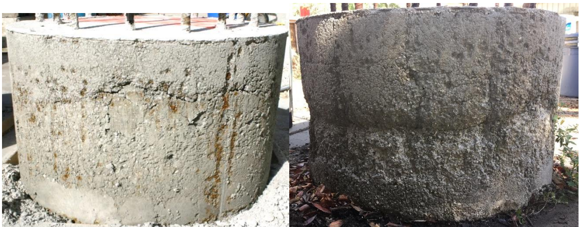
Figure 3.24 Shaft 24: Self consolidating concrete; 40 sec/qt bentonite; rough; disintegrating; creases coincide with deteriorated regions.
