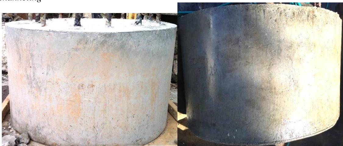
Figure 3.19 Shaft 19: f'_c 4100 psi; drilled shaft mix; 63 sec/qt polymer; smooth; no creases
