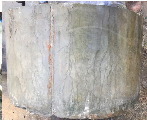
Figure 3.22 Shaft 22: f'_c 4100 psi; drilled shaft mix; water cast; smooth; faint channeling
