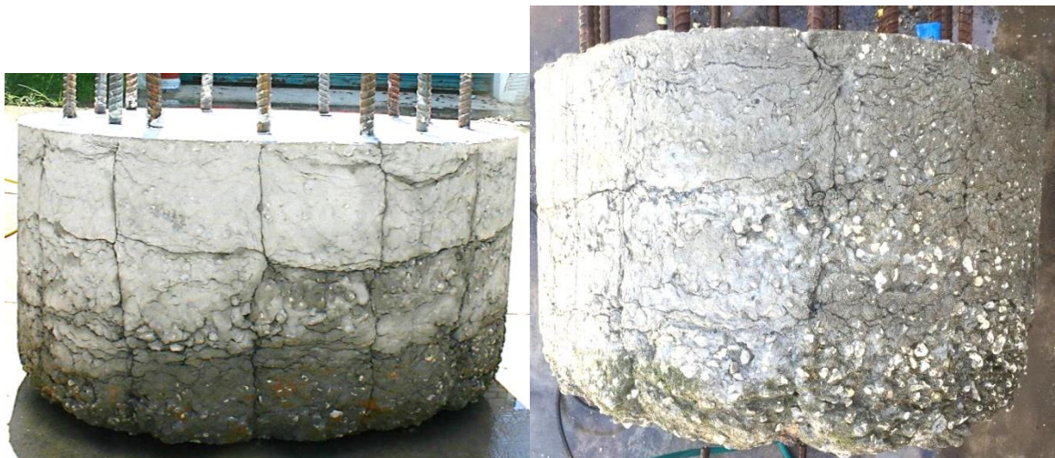
Figure 3.3 Shaft 3: f'_c 4358 psi; drilled shaft mix; 40 sec/qt bentonite; coarse; well-defined creases.
