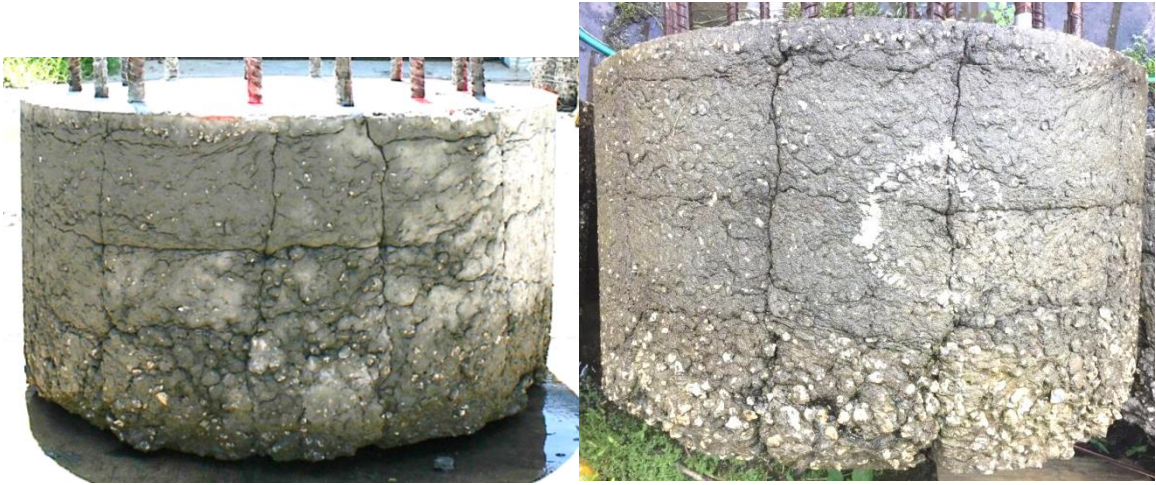
Figure 3.5 Shaft 5: f'_c 4358 psi; drilled shaft mix; 90 sec/qt bentonite; coarse; well-defined creases.
