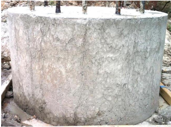
Figure 3.20 Shaft 20: f'_c 4100 psi; drilled shaft mix; 121 sec/qt polymer; smooth; faint creases.
