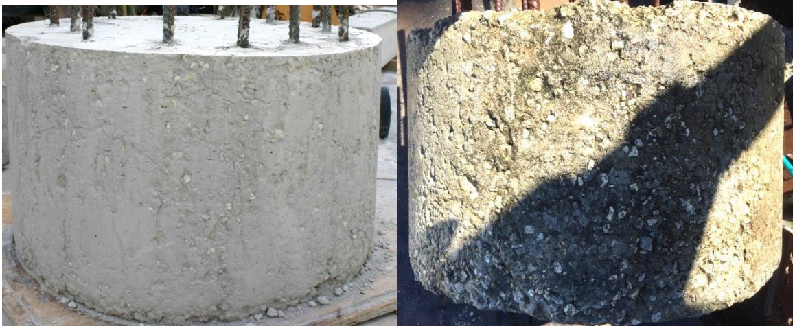
Figure 3.14 Shaft 14: f'_c 4753 psi; drilled shaft mix; 30 sec/qt bentonite; coarse; no creases
