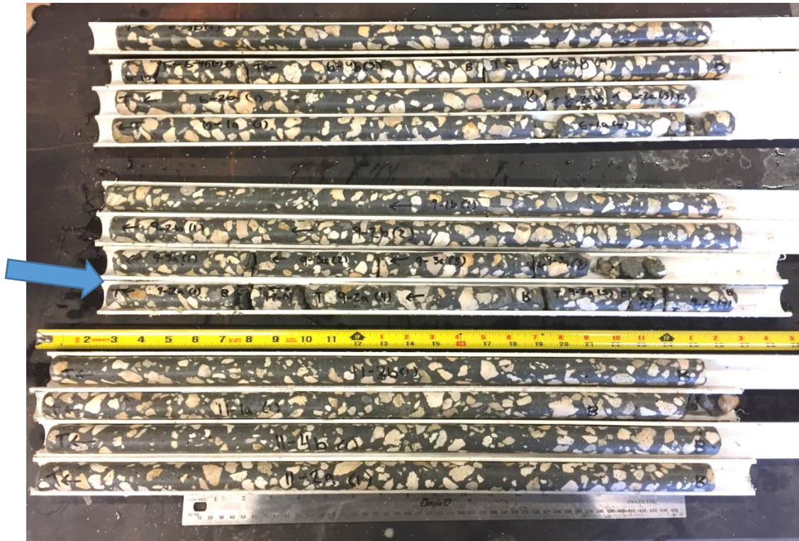
Figure 3.72 Core samples from shaft 11 (polymer), shaft 9 (bentonite), and shaft 6 (water)- (top to bottom).
