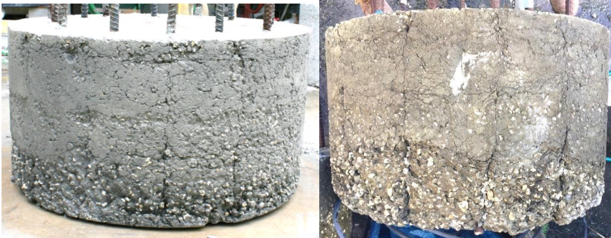
Figure 3.8 Shaft 8: f'_c 4530 psi; drilled shaft mix; 40 sec/qt bentonite; coarse; faint creases.
