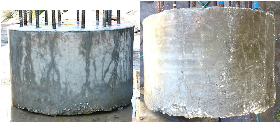
Figure 3.6 Shaft 6: f'_c 4358 psi; drilled shaft mix; water cast; smooth; faint channeling.
