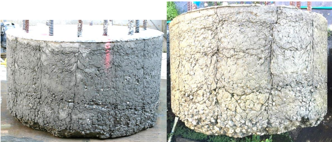
Figure 3.3 Shaft 3: f'_c 4358 psi; drilled shaft mix; 40 sec/qt bentonite; coarse; well-defined creases.
