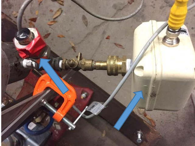
Figure 3.66-Pressure transducer and flow meter
