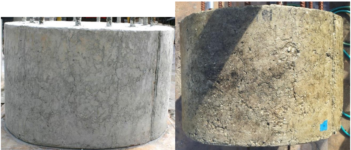
Figure 3.16 Shaft 16: f'_c 4753 psi; drilled shaft mix; 85 sec/qt polymer; smooth; faint to no creases
