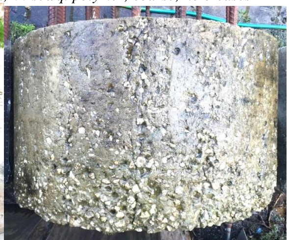
Figure 3.13 Shaft 13: f'_c 4753 psi; drilled shaft mix; 30 sec/qt bentonite; coarse; faint to no creases
