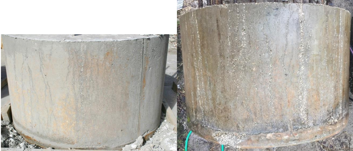
Figure 3.23 Shaft 23: Self consolidating concrete; water cast; smooth; faint channeling
