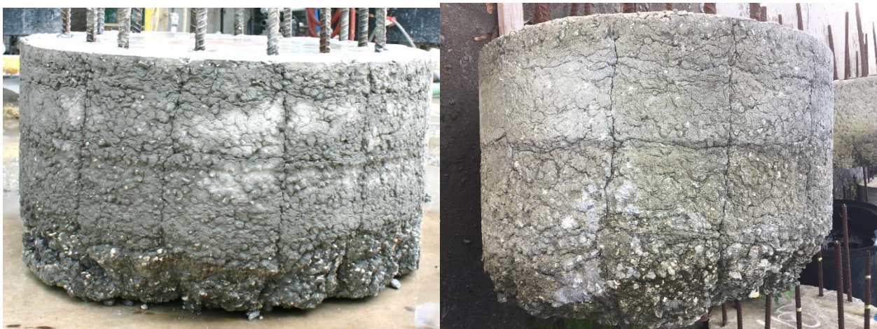
Figure 3.10 Shaft 10: f'_c 4530 psi; drilled shaft mix; 90 sec/qt bentonite; coarse; faint creases
