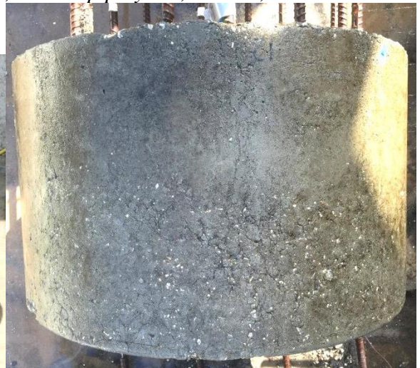
Figure 3.12 Shaft 12: f'_c 4530 psi; drilled shaft mix; 66 sec/qt polymer; coarse; no creases
