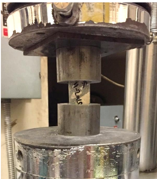
Figure 3.83 Core sample undergoing compressive strength testing
