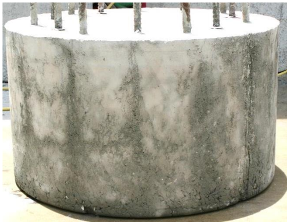
Figure 3.12 Shaft 12: f'_c 4530 psi; drilled shaft mix; 66 sec/qt polymer; coarse; no creases
