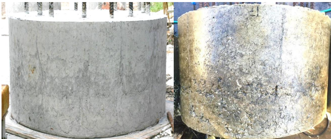
Figure 3.17 Shaft 17: f'_c 4753 psi; drilled shaft mix; 85 sec/qt polymer; smooth; faint creases
