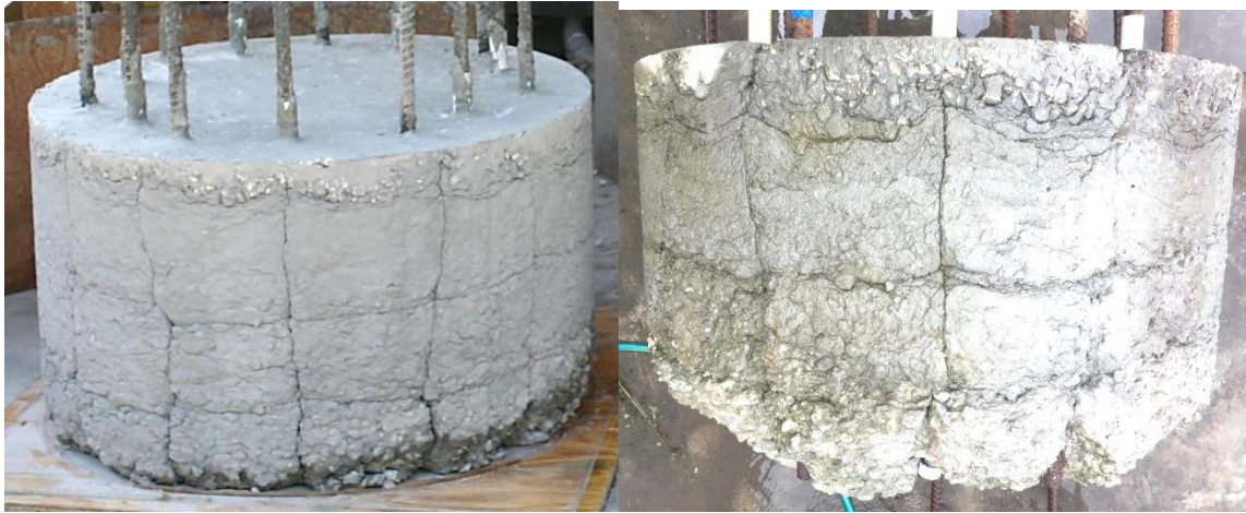
Figure 3.2 Shaft 2: f'_c 6150psi; drilled shaft mix; 105sec/qt bentonite; coarse; well-defined creases.
