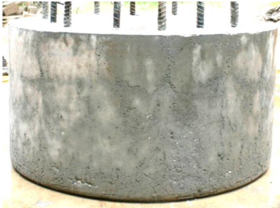
Figure 3.11 Shaft 11: f'_c 4530 psi; drilled shaft mix; 65 sec/qt polymer; smooth; no creases
