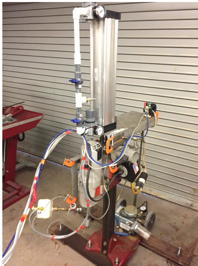
Figure 3.68- Instrumented, pneumatically controlled, core drill
