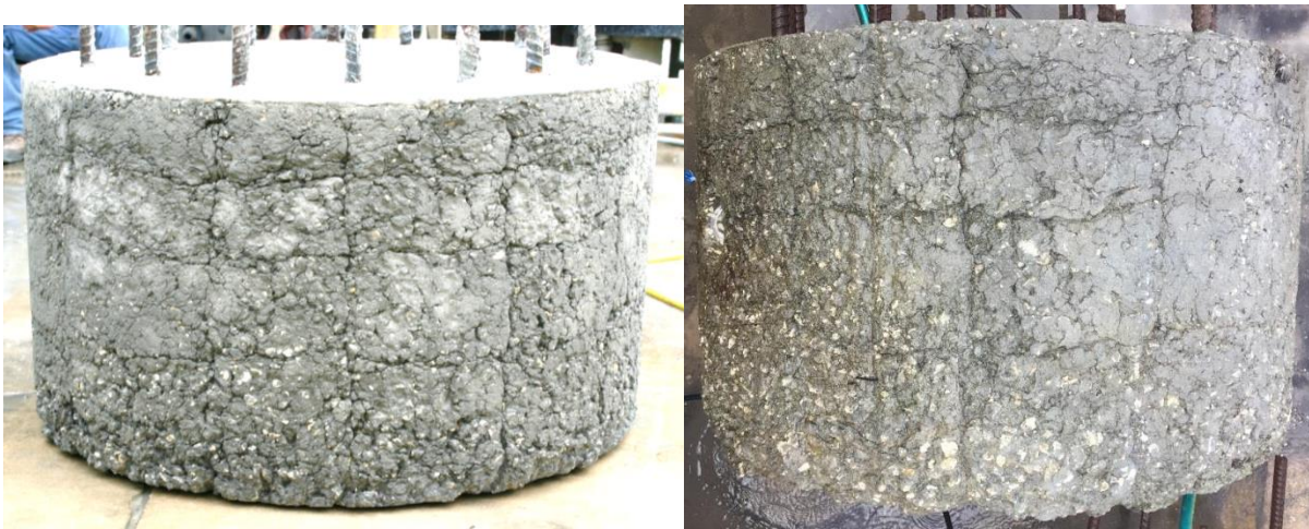
Figure 3.9 Shaft 9: f'_c 4530 psi; drilled shaft mix; 50 sec/qt bentonite; rough; with well-defined creases
