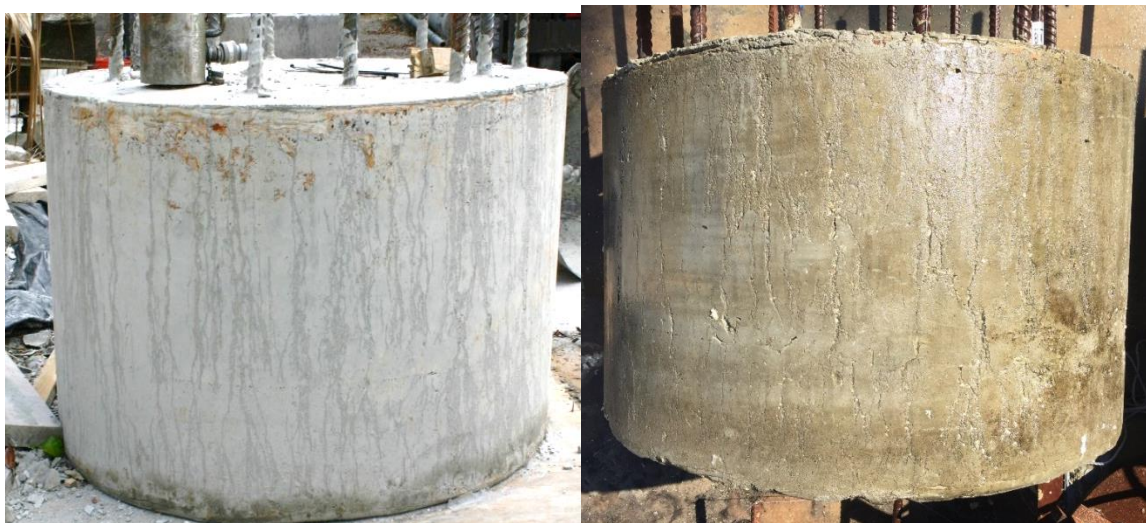
Figure 3.18 Shaft 18: f'_c 4753 psi; drilled shaft mix; water cast; smooth; faint channeling
