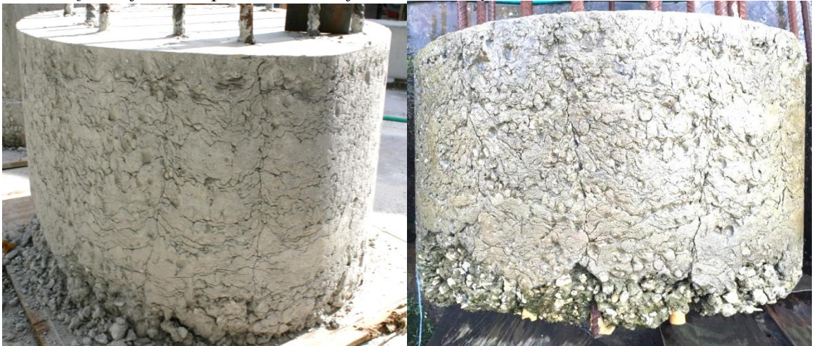
Figure 3.15 Shaft 15: f'_c 4753 psi; drilled shaft mix; 56 sec/qt bentonite; coarse; well-defined vertical creases
