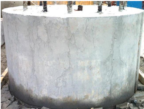
Figure 3.22 Shaft 22: f'_c 4100 psi; drilled shaft mix; water cast; smooth; faint channeling
